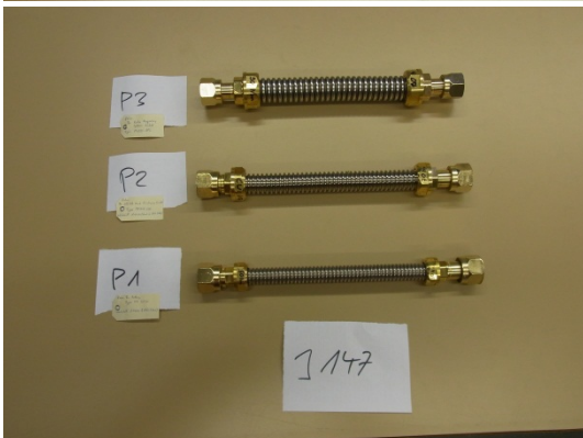
Figure 4: (before test start) Three different sizes were tested using different brands of corrugated tubes. P1: DN16 (Rattay HR I/S-W) P2: DN20 (Solar Kurt Birnbreier, MF015 500) P3: DN25 (Radio Frequency Systems, PW025-AFL)
