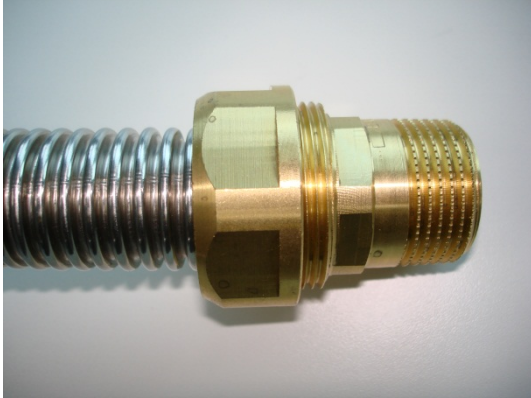
Figure 2: (before test start) Fast coupling system before tightening.
